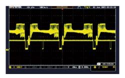
With respect to the waveform display technology, the GDS-1000B Series oscilloscope is capable of displaying 256 color gradients which can delineate the profound gradational fluctuations; as if it can recreate the analog oscilloscope display capability. When a multi-layer video signal is input, the GDS-1000B Series, with 256 color gradient display, has the ability to precisely reveal the
