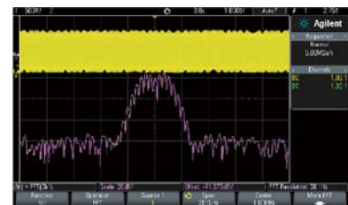
KEYSIGHT DSOX2000A - FFT Display
