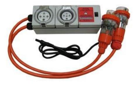
The PAC-TPL 3 phase leakage adaptor is now released. This adaptor provides users of the Seaward PAC3760 plus and Primetest Elite Testers with the capability of powering up 10A, 16A, 20A and 32A appliances and carrying out a leakage current test. The test results are displayed on the testers, with both the actual reading and a Pass/Fail display.
