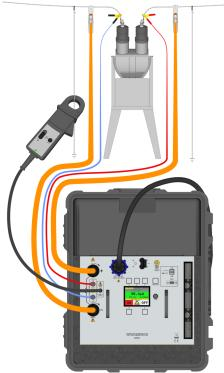
isolators and grounding links with both sides earthed are simple with the optional current clamp. This allows the current flowing through the earthing equipment to be subtracted from the test current.
