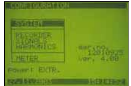
Configuration menu for setting measuring method, integration period, current scaling factor and selection of signals
