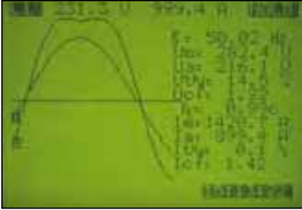
Scope function allows viewing of current and voltage waveforms
