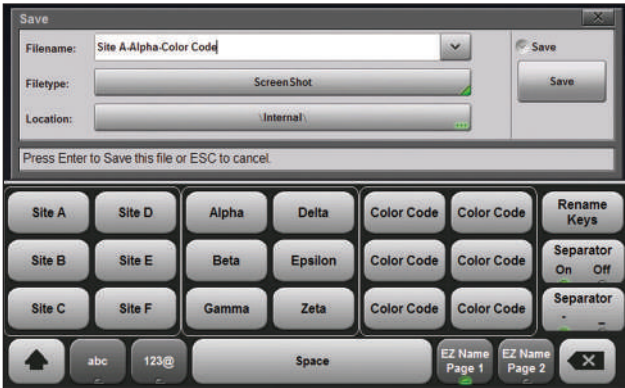
Most common site name requirements are preprogrammed into the EZ Name Matrix. Page 1 of 2 shown.
