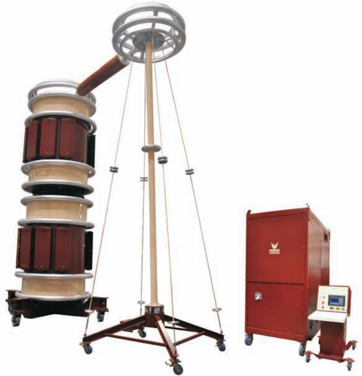
AC, Cascade Type, 400 kV, 800 kVA
